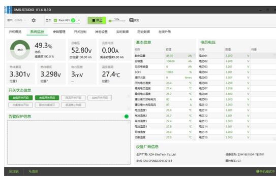
4.Choose to log in (password: 000000) to set some function settings such as operational parameters, inverter protocol switching (not recommended for terminal customers)
