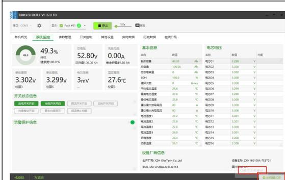
After the mode is switched to parallel mode, click Start to connect, and the interface has the data of each PACK
